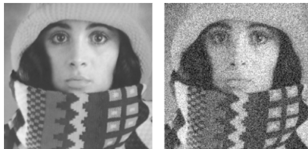
Figure 18.4. Input images for the filtering examples. Noise-free on the left (used in Figures 18.5 and 18.6), noisy on the right (Gaussian noise, SNR=4; used in Figure 18.7).
